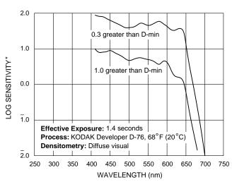
\*Sensitivity = reciprocal of exposure (ergs/cm²) required F002\_0511AC to produce specified density
