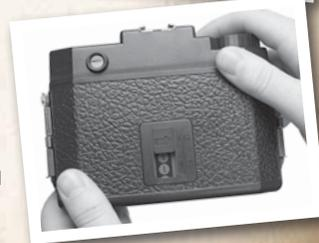
2. Open the back of the Holga. The exposed film should be in the film chamber on the right. An empty film spool will be in the film chamber on the left. Save the empty spool, as this is now the new take up reel for the next roll of film.
