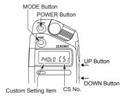
2. Press the UP or DOWN Button to select the desired custom setting number.
