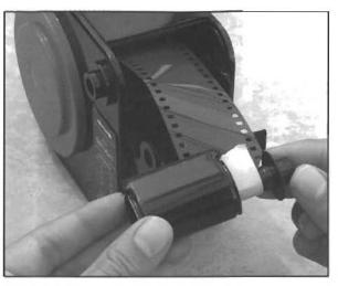
Slide cassette case over spool, with film extending through felt light trap.
