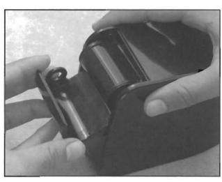
With the end ring of the cassette properly fitted against the light trap of the loader, close the door. Insert the crank, which engages the patented automatic lock and prevents film compartment door from opening. For the first few rolls loaded, keep loader on its side while winding to prevent scratches on film base.
