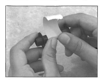
Loading bulk film with the Daylight Bulk Film Loader to the spool, allowing the ends to project.
