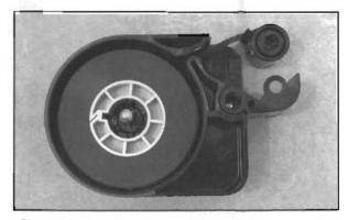
This "cut-away" view shows how cassette, loader and door fit together.
