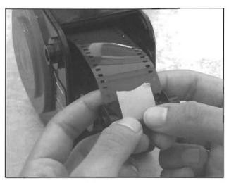
Place end of film against the spool, press one end of tape on top of film and the other end wrap around the spool and tape to the underside of the film. The tape is now looped around the spool and the ends attached to both sides of the film.
