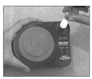
Hold the loader with the left hand and with your right hand wind the correct number of turns for the exposures you want in the cassette. The turns will vary somewhat with different spool diameters, as some are bigger than others. Generally, 36 exposures in a cassette equals 30 turns of the crank.
