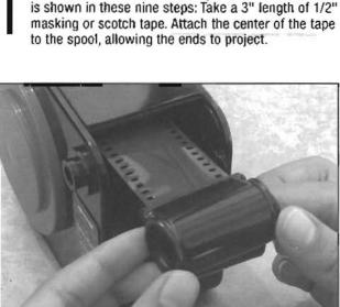
When using reloadable metal cassettes, put an end ring over the spool end and snap over the edges of the spool. Pull down lightly on the end and it will snap into place. Give the ring about 1/8 of a turn to see that it is properly seated into the groove.
