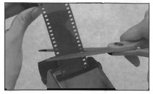
Next, remove the crank from the loader, open the door and take out the cassette. Pull an additional 3-1/2" of the film from the loader for use as a leader when loading the film in the camera. Cut off the film from the bulk roll between the sprocket holes.
