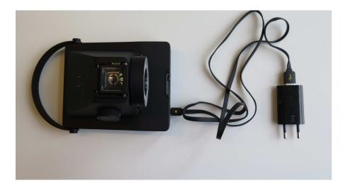
4. Disconnect the Impossible I-1 USB cable from the Impossible I-1. Double check that all switches are on the positions explained on step 1 (Camera: OFF, Flash: ON, Lighten/Darken switch: MIDDLE)
