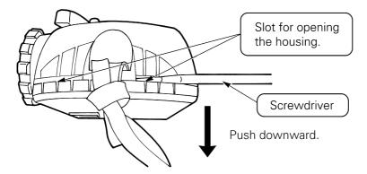
2. After removing the rear cover, insert the screwdriver into the slot on the side opposite the strap and lift up the main unit.
