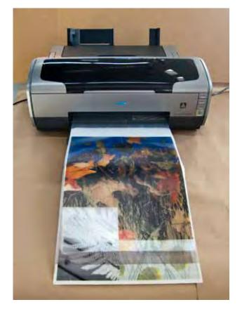
8. Before printing run a nozzle pattern check to make sure the printer is printing properly. This will keep from wasting the custom substrate.
