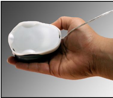
Positioning basICColor SQUID2 for ambient light measurement.
