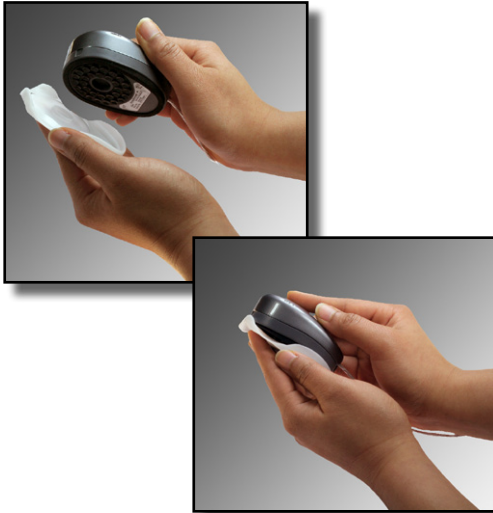
Mounting the ambient light head on a basICColor SQUID2
