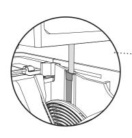
Insert the probe into the probe slot and close the lid by pushing it towards the tank like the standard lid.
